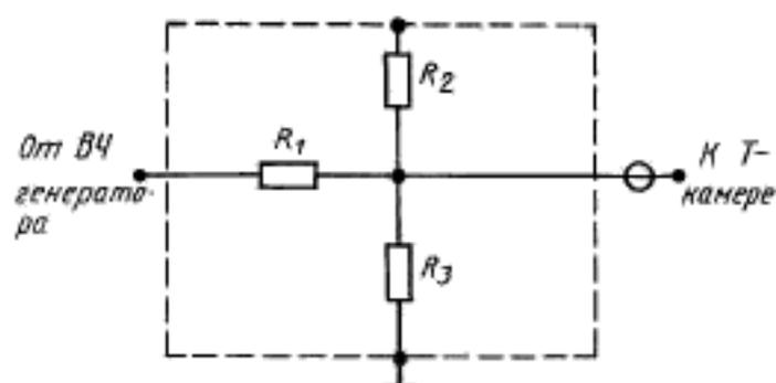
$$R_1 = R_2 = R_3 = 122,5 \text{ Ом}$$
